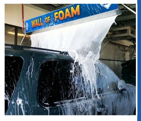
When used as a foaming arch it utilizes three separate foam generators that adjust the amounts of chemical, water, and air to get the desired foam wetness and the consistency you want. The arch can come with custom graphics that are tailored to your car wash allowing you to promote your brand, a specific use, or a new car wash package.
