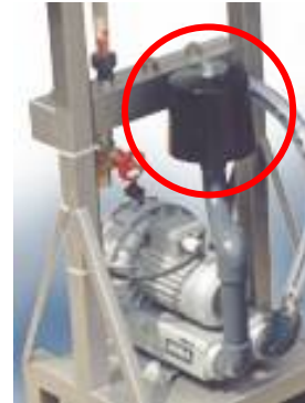
Figure 7-1 Air intake filter
